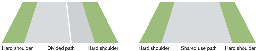
The purpose of divided paths and shared use paths is to improve conditions for cyclists and pedestrians on stretches without infrastructure for vulnerable road users by ensuring that they get areas/routes of their own, separated from vehicular traffic. Typically, the measures are constructed as paths in their own layout and are used on roads with few cyclists and pedestrians and with limited space, and thus being difficult to construct cycle track and pavement.
